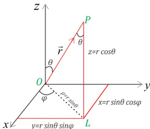
Figure 4.1: Rectangular to Spherical Coordinates
